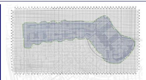
This scheme was undertaken to infill the 'Red' coal seam, at 22-28m depth, over the entire development area (as shown on the grid layout plan above) and to treat one located mineshaft which was around 70m deep. Overlying superficial deposits were up to 20m deep requiring the use of specialist geotechnical rigs and drilling techniques. 5 drilling rigs were resourced to site.
